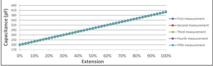
Extension (%) = Extended Sensor length / Original Sensor length\*100% Repeatability: <±1%
