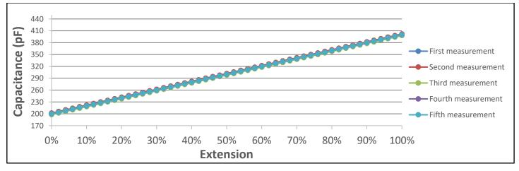
Extension (%) = Extended Sensor length / Original Sensor length\*100%
